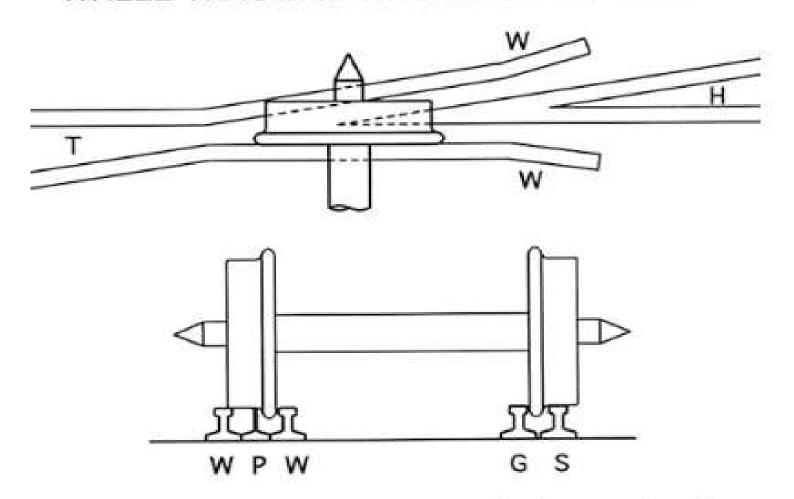
P = point of frog W = wing rail S = stock raill G = guard rail T = toe H = heel
