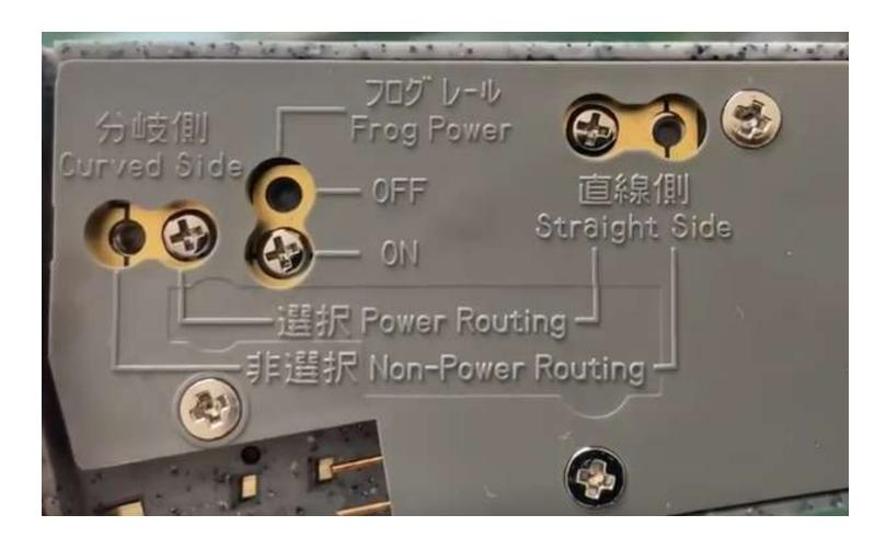
Digitrax and other DCC manufacturers recommend setting Kato #4 turnouts to non-power routing for better DCC performance.
