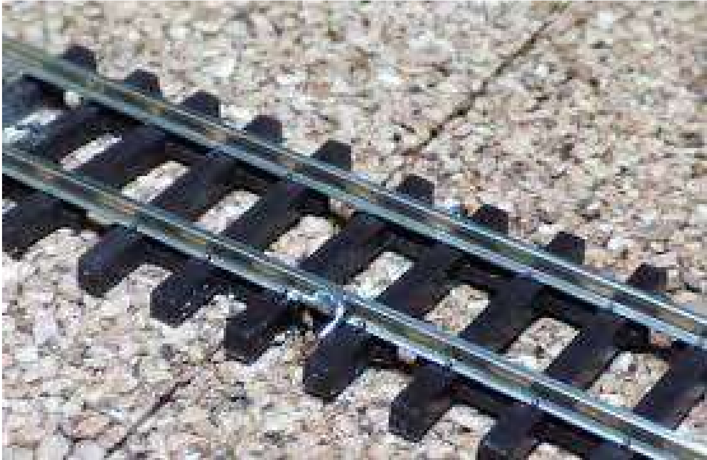
Soldered Solid Wire to Rail Outer Rib
